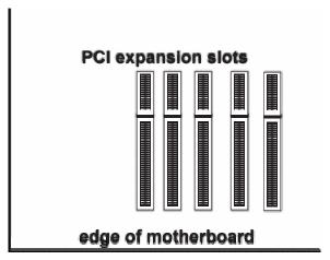
Insert the ADAC Ultra2 S466 card in a PCI slot as shown below:
